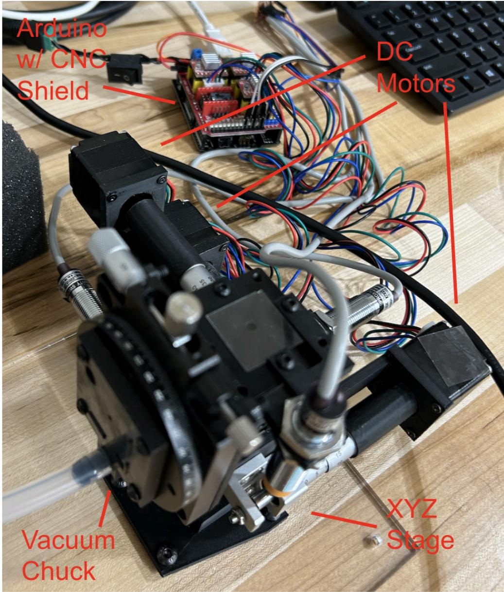
**Figure 6.** Assembled XYZ stage.
