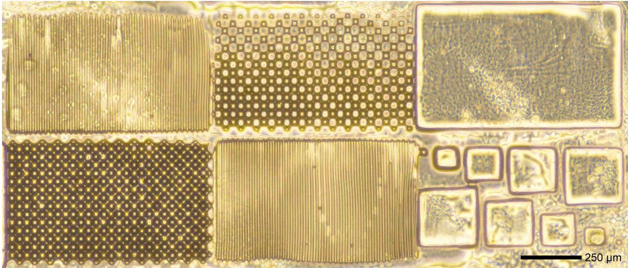
**Figure 20.** A multi pattern etch showing off the pattern changing and tiling functions
