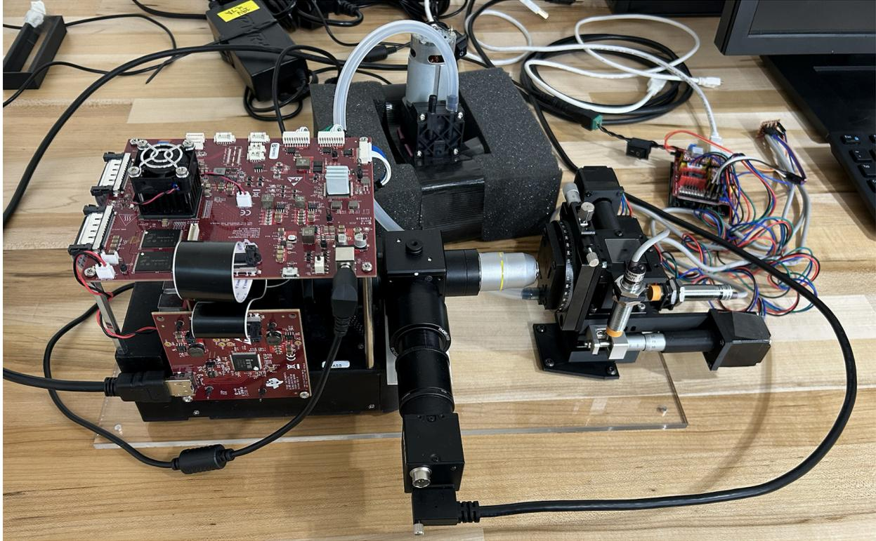
**Figure 7.** Complete photolithography stepper assembly.
