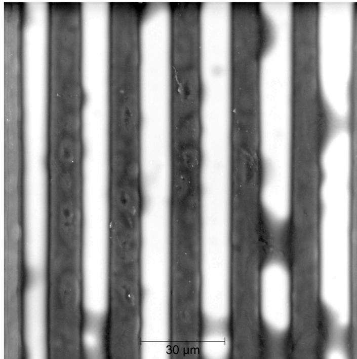
**Figure 21.** Fine line exposure under BSD SEM
