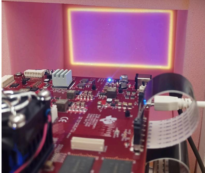
**Figure 4.** UV swapped projector showing a “blue” screen with a board.
