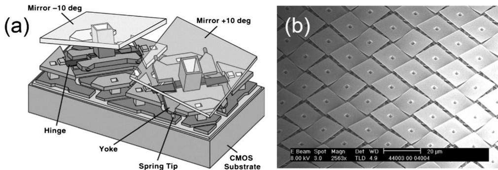
**Figure 1.** (a) DMD elements and (b) top-down view of landed DMD mirror array [7].
