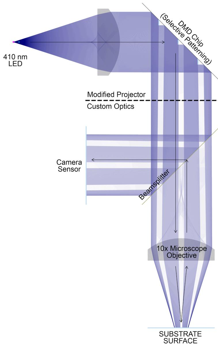
**Figure 2.** Diagram of photolithography stepper assembly.
