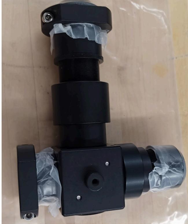
**Figure 5.** Assembled optical train for photolithography stepper, sealed with parafilm.
