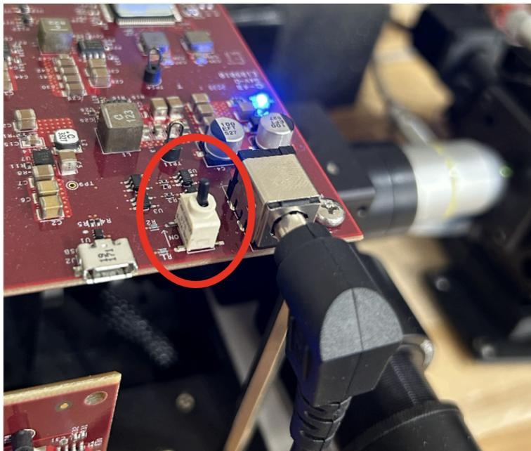
**Figure 11.** Projector power switch in "on" position
