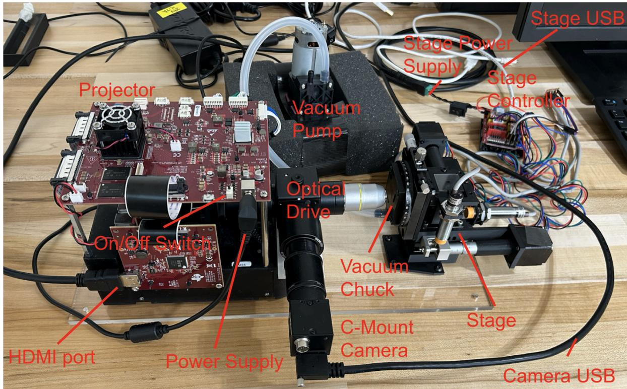
**Figure 10.** Labeled Photolithography Stepper
