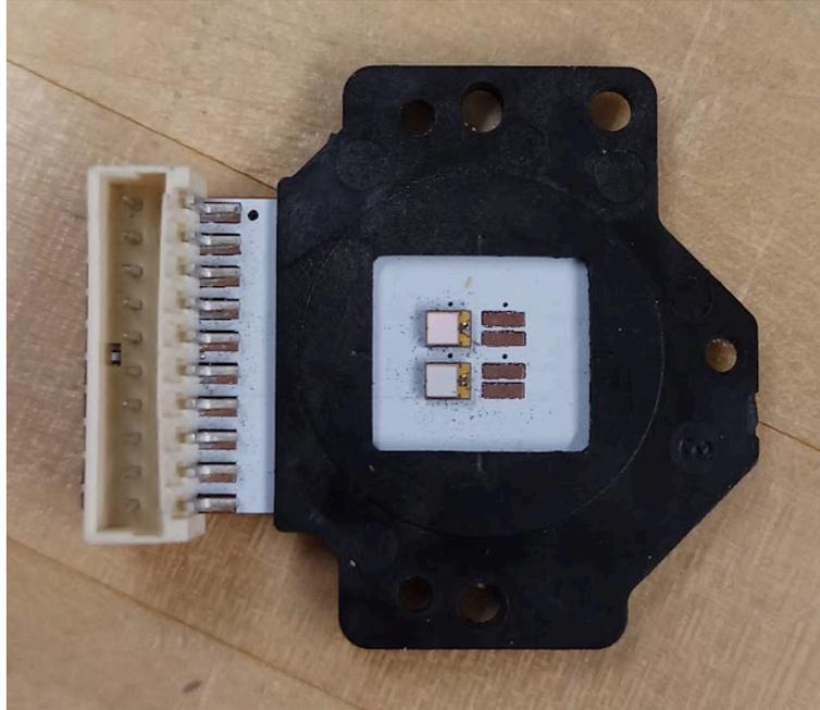
**Figure 3.** Custom UV LED board for replacement in DLP projector.
